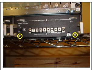
Removal of the top metal cover on PEM A and PEM B requires a T9 Torx Screwdriver.
