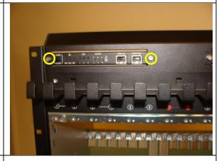
Removal of the shelf alarm display combiner board requires a Torx T10 screwdriver.
